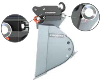
Safely locked. Indicator pin is driven in.
